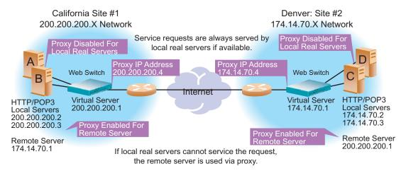
Figure 12-4 POP3 Request Fulfilled via IP Proxy
